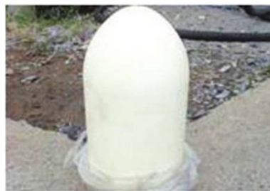
PIG FOR COLLECTING PRODUCT(BEFORE PIGGING)
