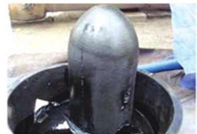
PIG FOR COLLECTING PRODUCT(AFTER PIGGING)
